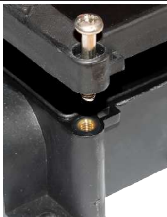
1: Four captive stainless-steel screws tightening on metal inserts. No screwing into the plastic, no fragile hinges.
