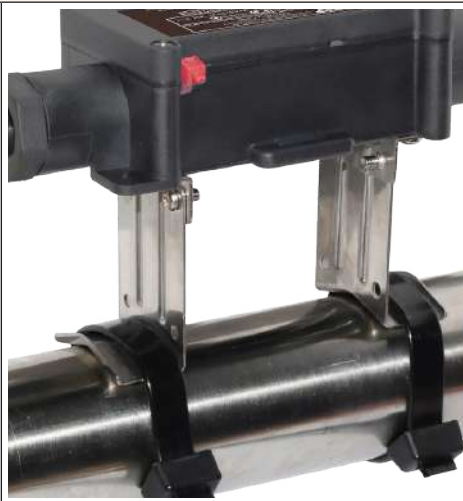
3: One stainless steel bracket , for offset mounting on piping , allowing the enclosure to be locked in after the insulation and its protection have been installed. Allow an insulation thickness of 50mm , and can be used on hot pipes. Clamping on metal or PVC piping by nylon tie or metal clamp. (Legs available as an accessory.)
