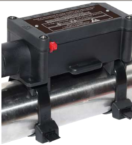
2: Two removable PA66 plastic tabs , for fitting on pipes , providing a 10mm offset from the tube. Ideal and economical for applications with low insulation thickness and pipe temperature below 100°C. Clamping on metal or PVC piping can be made by nylon tie or metal clamp (These tabs are included as standard).
